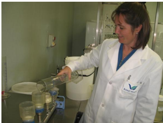
Figure 3-4(L3) Vacuum manifold fitted with 47mm membrane filter holders
