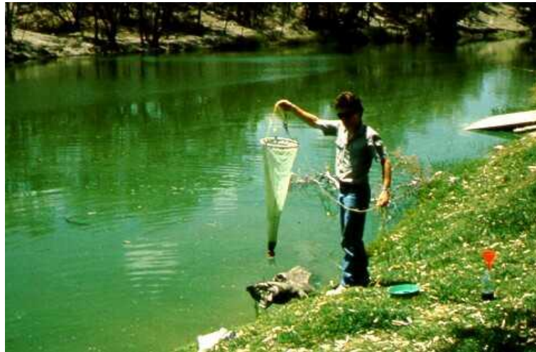
Figure 3-5 Net sampling is a simple method for concentrating cyanobacteria for further analysis
