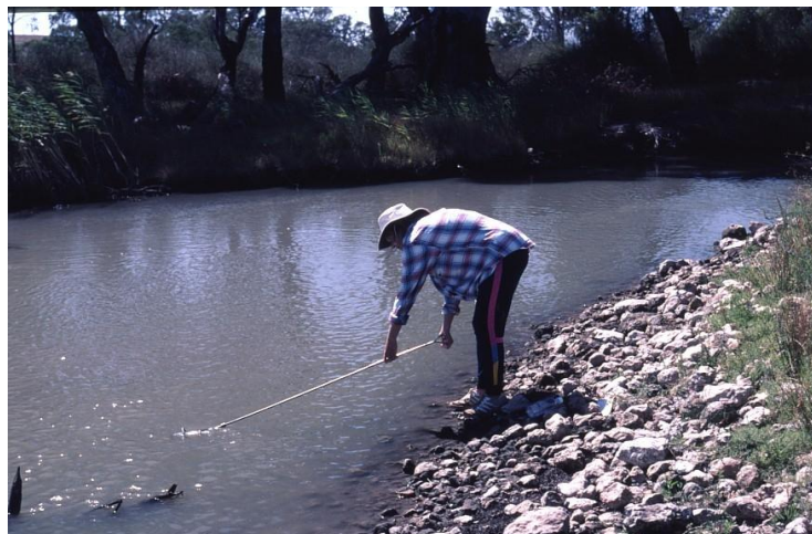
Figure 3-4 Taking grab samples from the shoreline with an extension pole.
