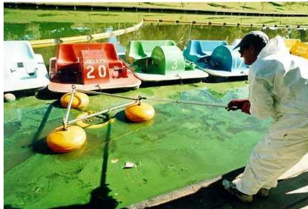
Figure 4-3 The use of a skimmer to remove surface scum in a recreational lake in South Australia. Toxic material was collected and disposed to sewer
